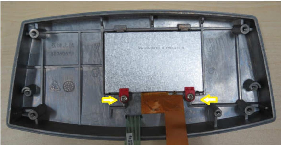
Location of the 2 screws holding the TFT in place against the Terminal Top housing. (Note the position of the two RED holders)
