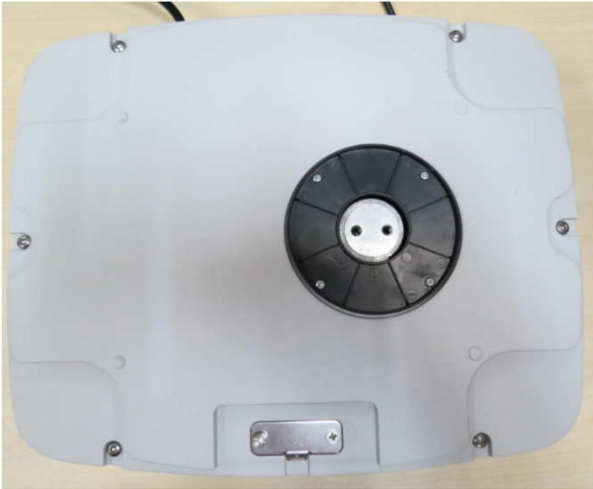
Spider removed from base top housing.
