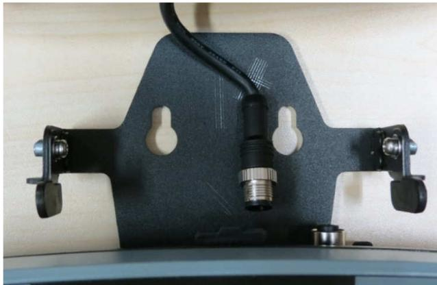
2. Removing the docking bracket from the Terminal.
