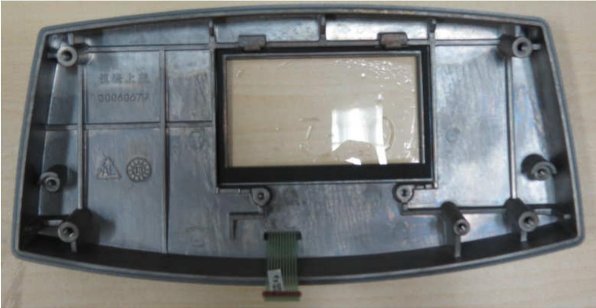
TFT PCB removed from Terminal Top housing.
