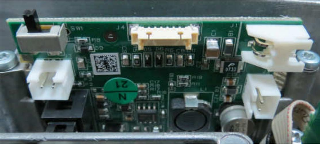
Picture shows 5 cables removed, location of the 2 screws.
