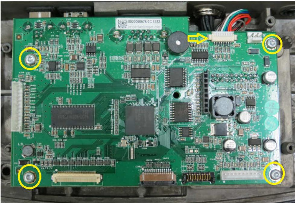
Location of the 4 screws and 8PIN connector on the Terminal PCBA.
