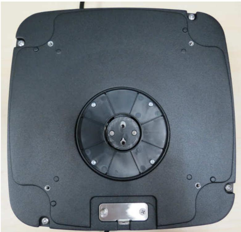
Spider removed from base top housing.
