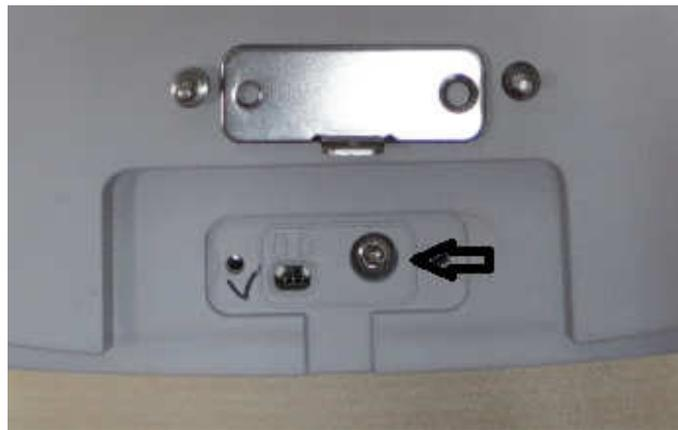
7<sup>th</sup> screw expose, by removing this screw you will be able to dismantle the base top housing from the base bottom housing.
