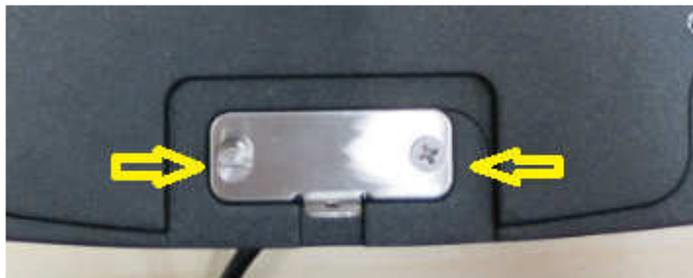
Remove the 2 screws securing the LFT cover.
