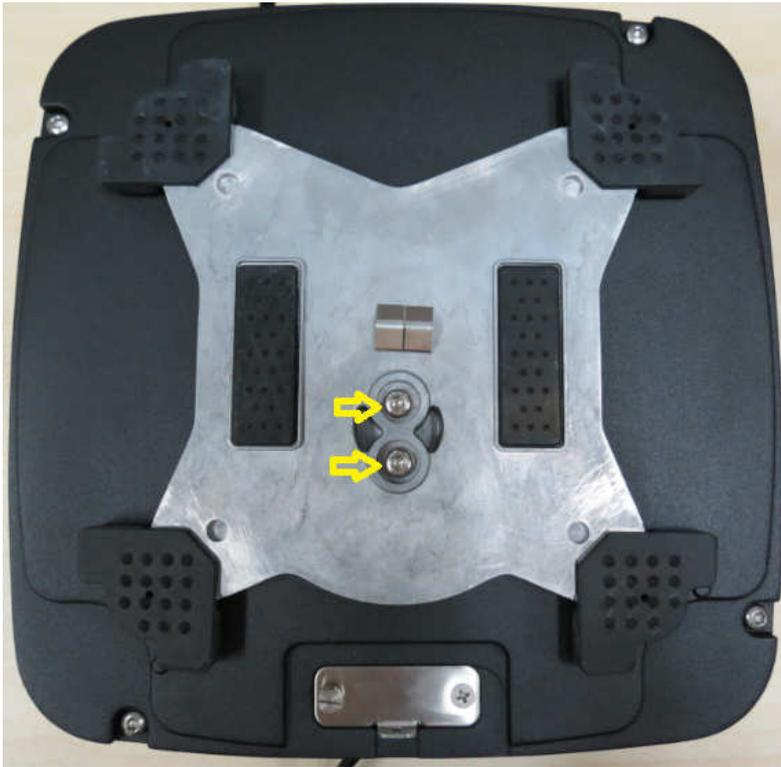
Location of 2 screws securing the Spider with base top housing.
