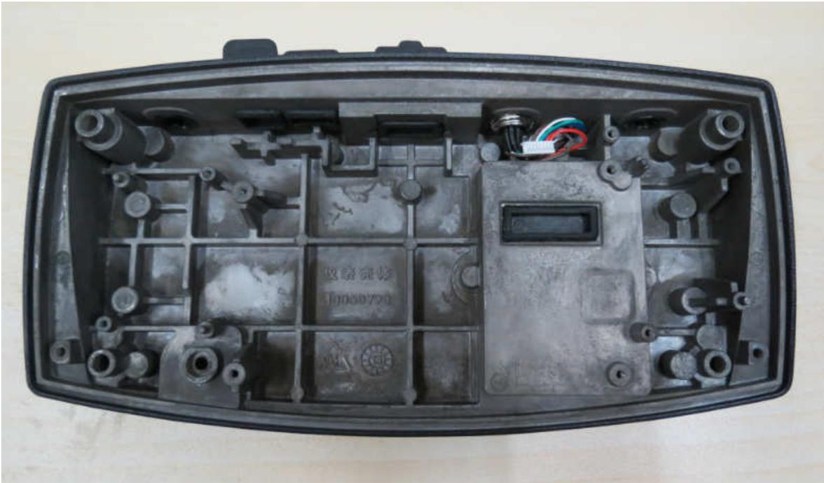
Terminal PCBA taken out from Terminal bottom housing.
