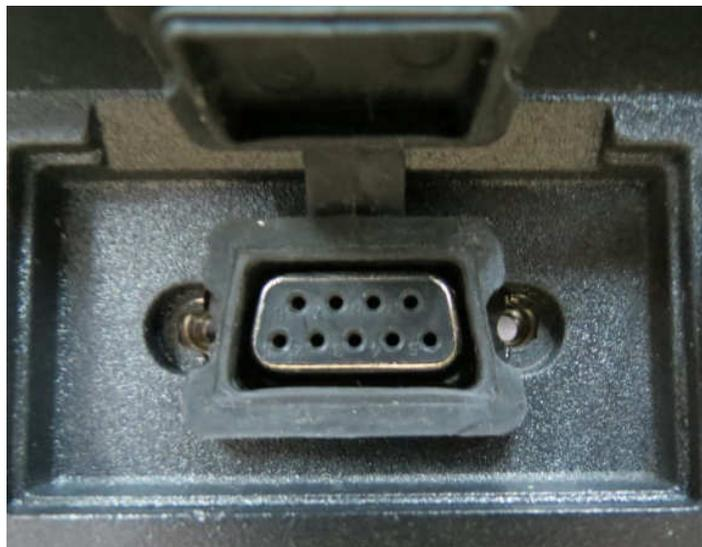
2 screws securing the RS232 port against the Terminal housing removed.
