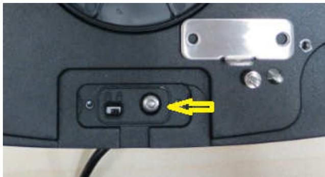
5<sup>th</sup> screw expose, by removing this screw you will be able to dismantle the base top housing from the base bottom housing.
