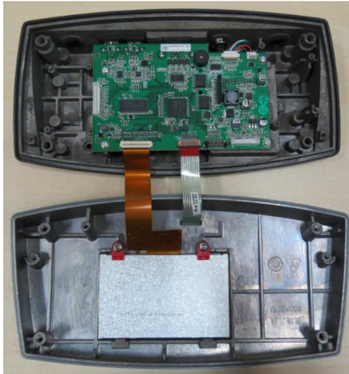
3. Disconnect the ribbon cable connecting the TFT with Terminal PCBA by using a thin screw driver blade radiated the back cable-lock on the connector 90° so that it is perpendicular to the cable as show in below pictures.
