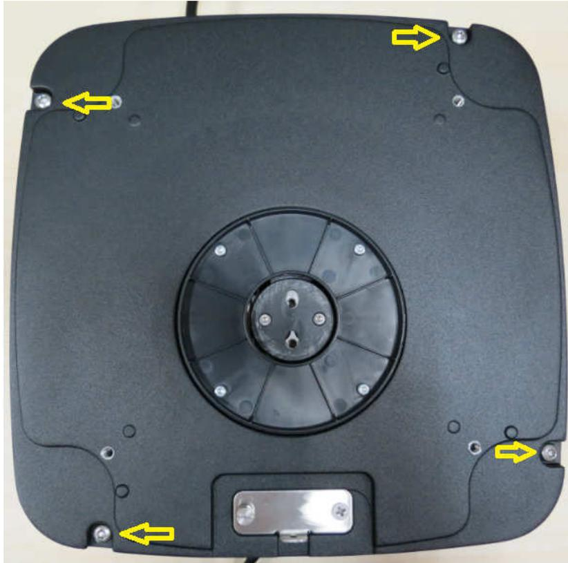
10. The 5<sup>th</sup> screw is underneath the LFT cover.
