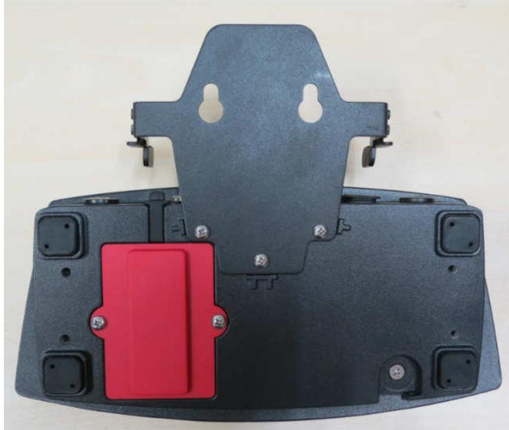
3. Flip the Terminal around locate the 3 screws as shown and remove the screws which are mounting the bracket to the Terminal as shown below and separate the docking bracket from the Terminal.
