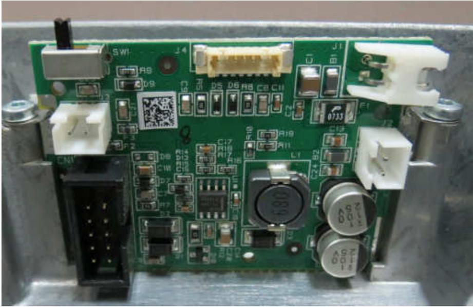
Picture shows 5 cables removed, location of the 2 screws.
