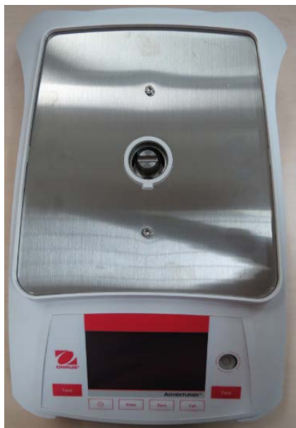
Figure 3-21 Adventurer Precision balance Pan Support removed.
