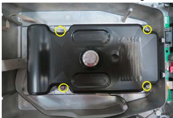
Figure 3-30 4 screws holding the cell to the balance bottom housing.
