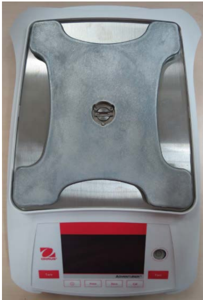
Figure 3-20 Adventurer Precision balance with weighing pan removed.
