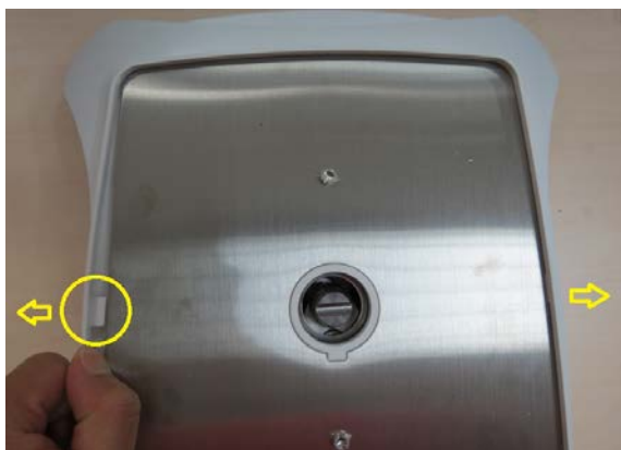
Figure 3-22 Adventurer Precision Balance Releasing hinges.
