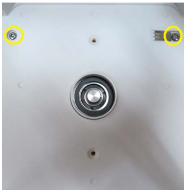
Figure 3-5 Analytical Draft Shield screws location.
