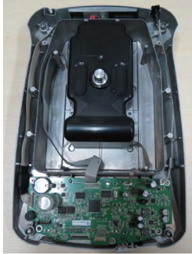
Figure 3-27 Adventurer Analytical Load cell metal cover removed
