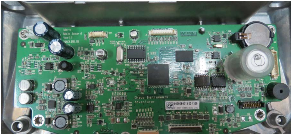
Figure 3-38 Two cables removed from main PCBA.
