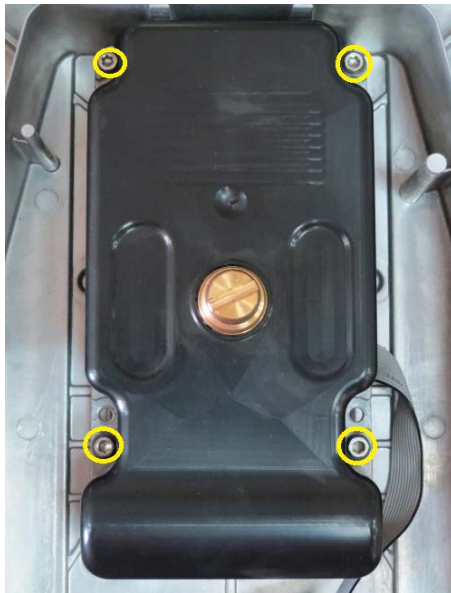
Figure 3-35 Location of the 4 screws securing Strain Gage load cell to the balance bottom housing.
