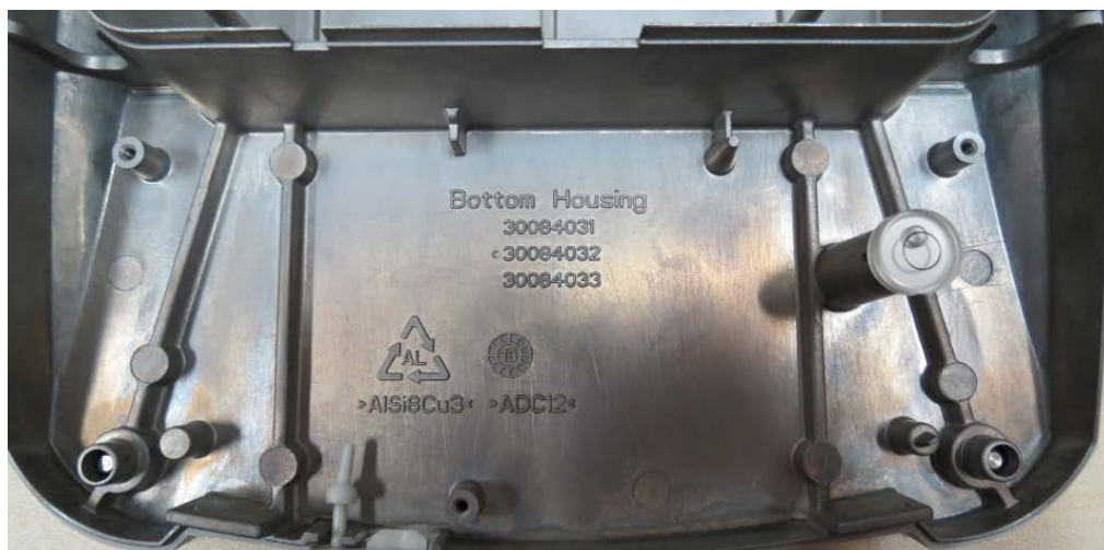
Figure 3-40 Main PCBA removed from bottom housing.
