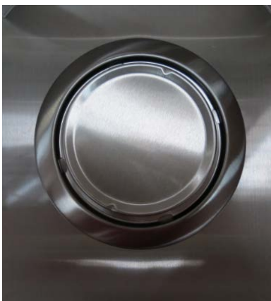
Figure 3-1 Analytical Weighing Pan and Wind Ring attach.
