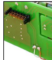
Figure 3-70. Solder points on Position Sensor Board.
