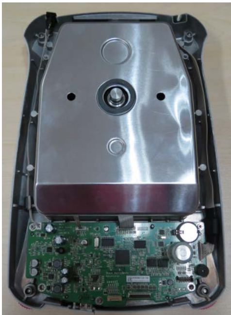
Figure 3-18 Adventurer balance bottom housing with top housing removed.
