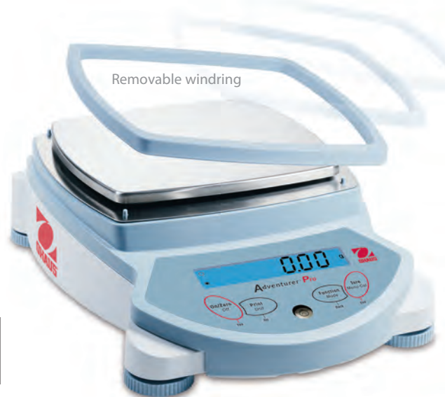
1mg models include draftshield
