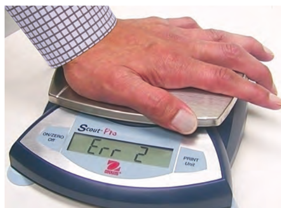
Mechanical and software overload protection
