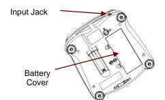
Connect the AC Adapter plug to the input jack.
