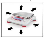
Avoid excessive air current, vibrations, heat sources, or rapid temperature changes.
