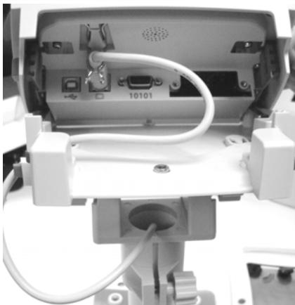
Insert the cable plug with the security clip open, then press the security clip into position to secure the cable.
