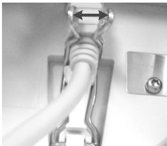
Release the clip that secures the Display Communication Cable: press out on both sides, as shown.
