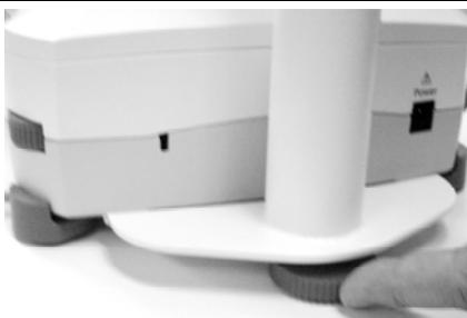
Re-connect power to the Base. Use the Level Assist feature to re-level the Balance. (Keep the Tower foot raised during this procedure.)
