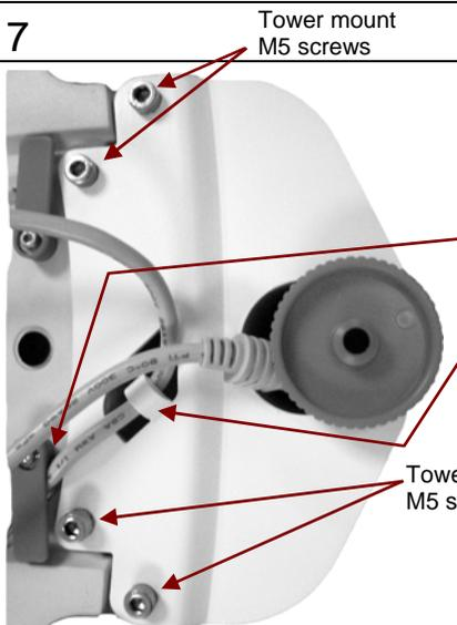
Attach Tower to the Base using the four M5 screws and wrench (supplied).
