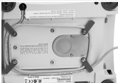
Un-spool the Display Communication Cable from the base.
