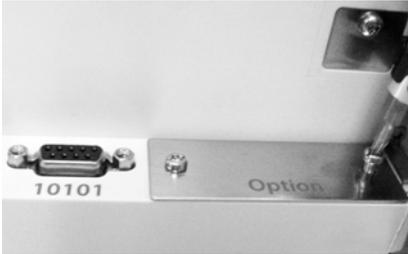
Remove the two screws holding the **Option** faceplate using a screwdriver. Remove this plate. Save the screws, they will be used to install the new RS232 interface board.
