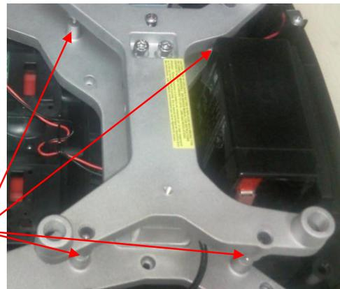
Figure 3-5. Overload Stops.
