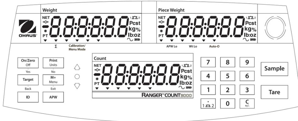
Figure 1-1. Ranger Count 3000 Front Display with controls.
