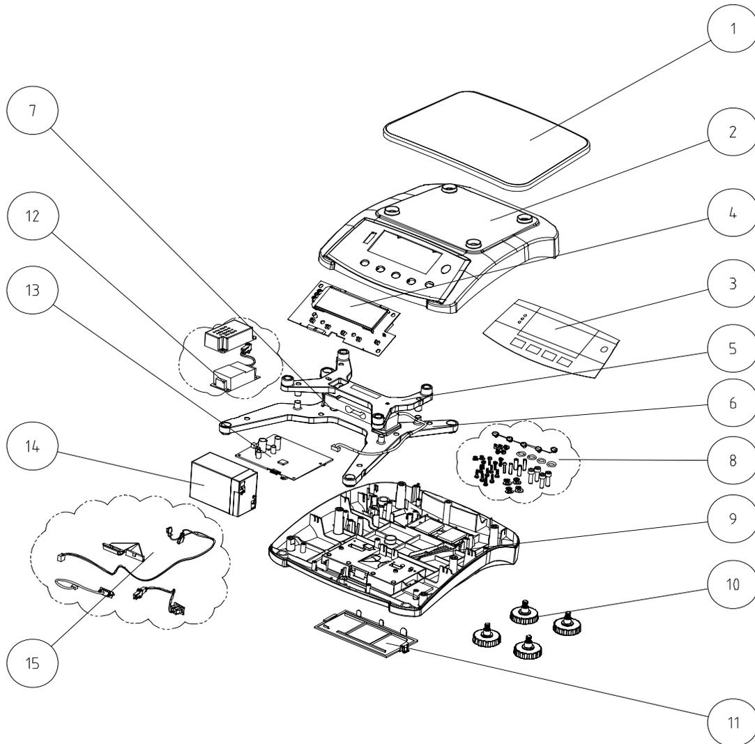
Figure 5-1. Ranger 3000 Scales: Parts.
