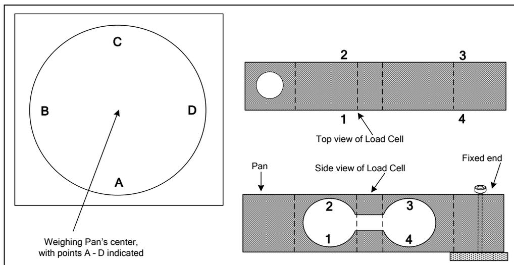
Figure 4-1. Scale drawing of Ranger 3000/Ranger Count 3000 Load Cell and Weighing Pan.
