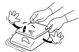
Take the battery out when scale is not in use for long time. Leakage from the batteries is hazardous.
