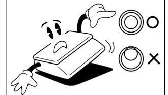
Keep the scale away from other electromagnetic generating devices. This may interfere with accurate reading.
